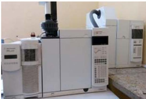
Plate 1: Gas Chromatography Mass Spectrometer Detector
