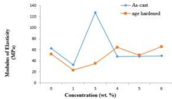
Figure 7. Plot of modulus of elasticity against concentration of banana stem particles
