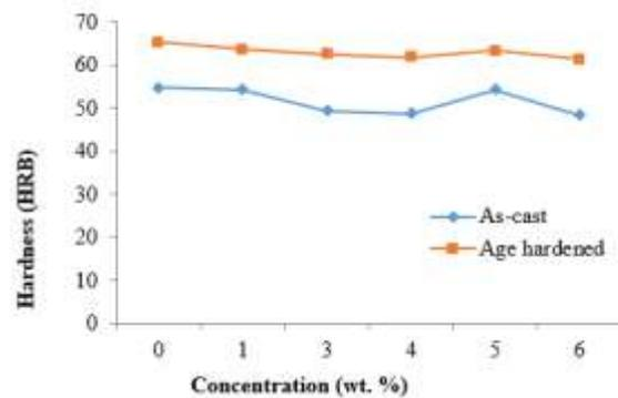
Figure 4. Plot of hardness against concentration of banana stem particles
