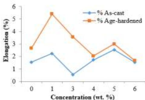
Figure 6. Plot of elongation against concentration of banana stem particles
