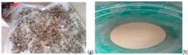
Figure 2. (a) Dried banana stem flakes (b) particles obtained from flakes after grinding
