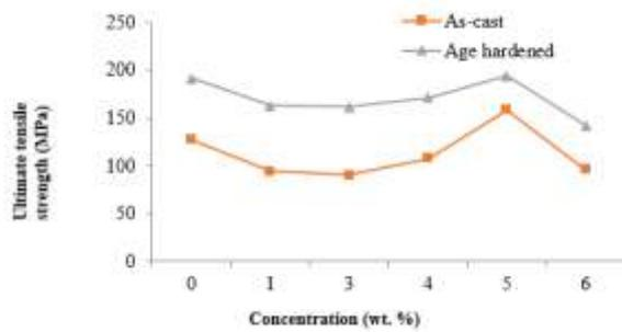
Figure 5. Plot of ultimate tensile strength against concentration of banana stem particles
