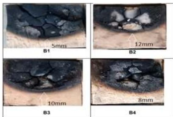
Figure 7: Test samples after fire test showing extent of flame propagation
