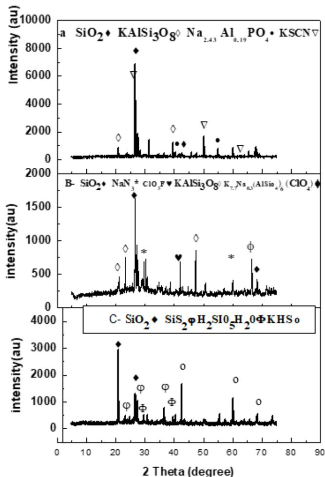
**Figure 6:** XRD patterns of the combustion of (wood, coconut husk and kaolin burned ratio) on the ash yield (a) Run 22, (85 %-5 %-10 %) (B) Run 21 (50 %-45 %-5 %) (C) Run 9 (5 %-95 %-0 %)
